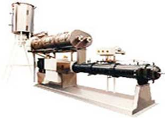
MEGA-TCX-80 Upto 1 TPH Cap. (Twin Screw with Preconditioner & Live Bin)
