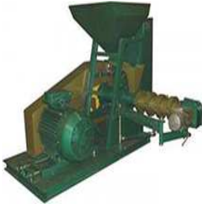
Single screw extruder for full fat Soy flour, corn + wheat, etc.
