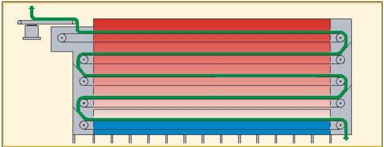
Schematic diagram of multi-pass belt drier used in instant food production line
