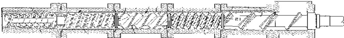
Fig 4) Screw & Barrel segments of Extruder for Aquafeed pellets
