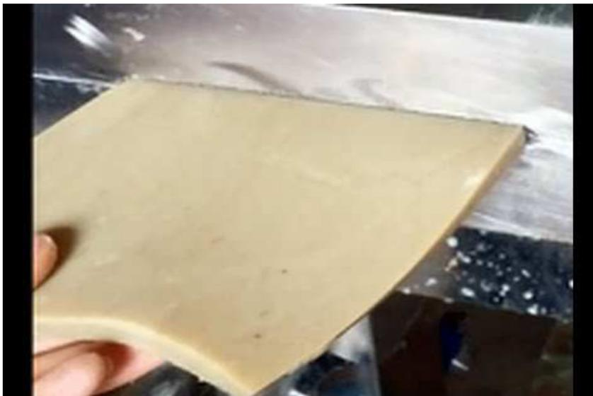
**Fig.3 .The Trial product emerging through the Slot Die.**
