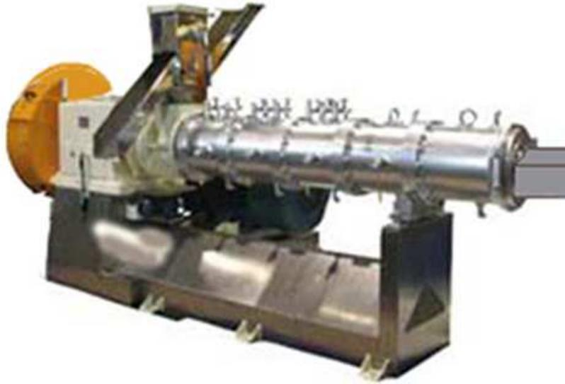
Single Screw Extruder for producing HMMA products.
