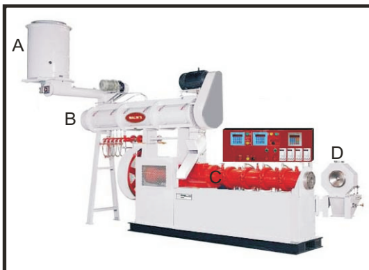
Extruder unit for floating feeds 300 Kg/h
