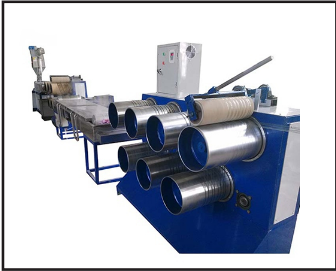
MEMFseries Extruder for producing PET, PP, Nylon, PBT monofilaments and synthetic hairs
