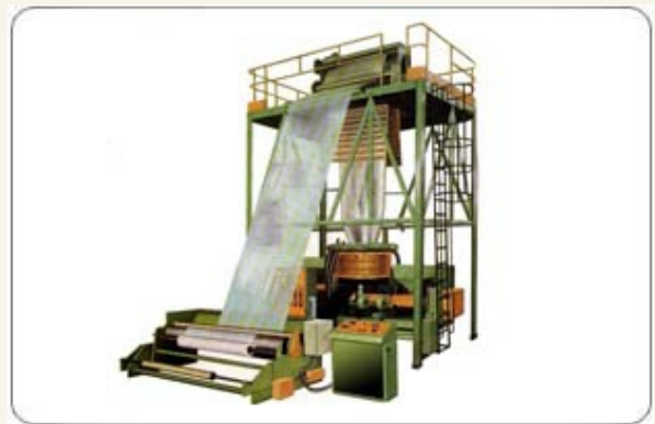
MELHM- Mono layer Film, Tubing, Rolls, liner from LDPE,LLDPE,HDPE,HMHDPE,PVC,PP, also Biodegradeable Bags.
