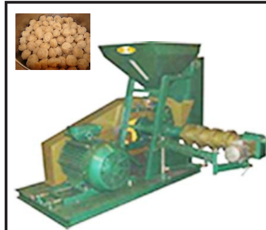
Extruder for Expanded Soy Chunks from Defatted Soybean grits. Can do full fat Soy too.
