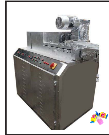
MEFEBG series Twin Screw Extruder for Sweet Bubble Gum
