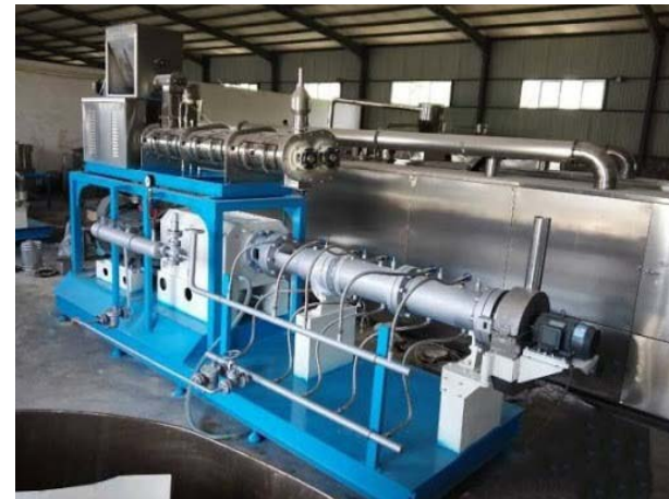
MEGA TX-65 Twin screw Extruder with preconditioner for producing floating Aqua pellets and other pet food
