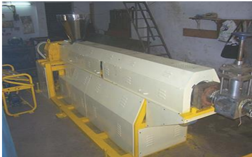
T-Die with 3 layer Feed block & Screen changer & CO2 foaming panel
