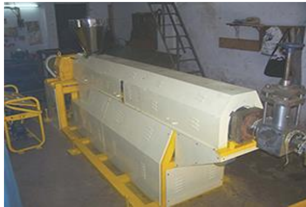
CO2 Foaming base Single screw Extruder for producing LDPE liners for wads.
