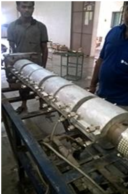
CO2 Foaming base Single screw Extruder for producing LDPE liners for wads.
