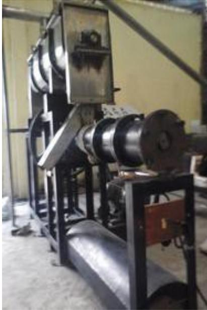
Medium Shear Extruder for producing Race Horse feed pellet
