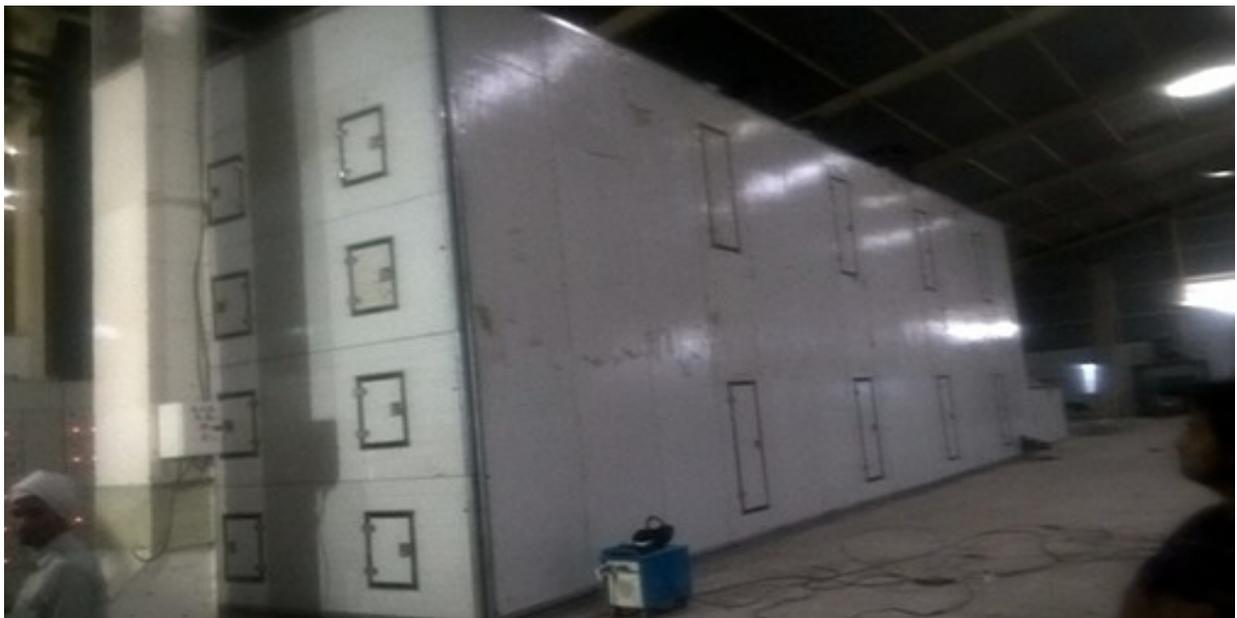
Pasta products Drier 7 Layers- 2 Tons/hour Drying Capacity of product
